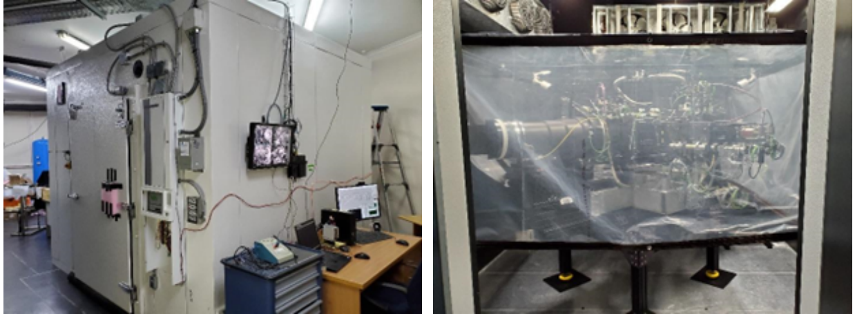
Figure 1. The NIR enclosure in the SALT Spectrometer Room (left) and the instrument inside (right). The fiber cable will enter the enclosure through the rectangular hole (currently filled with pink foam) in the upper left corner above the door. The plastic shroud around the spectrograph is to shield optical components from direct air currents from the cooling system.
