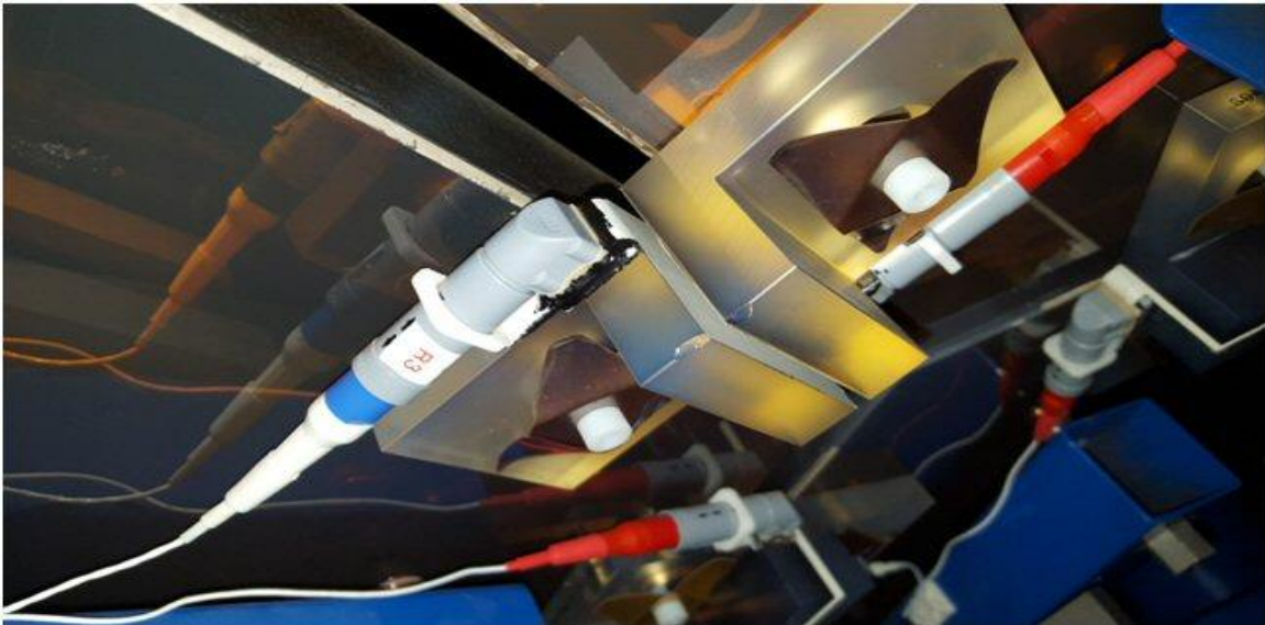
Fig: Inductive edge sensor mounted to the underside of a SALT Primary Mirror segment
