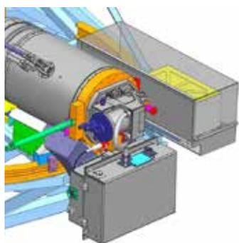
The new RSS detector shown on the end of the RSS camera barrel. The large enclosure underneath is a concept for mounting the CCD controller.
