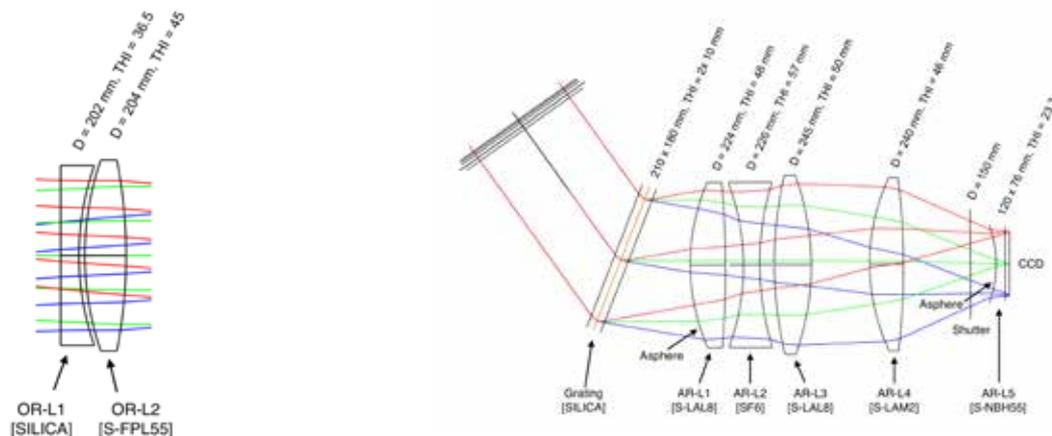
Figure 1: Optical layout of the Red collimator doublet (left) and camera (right).
