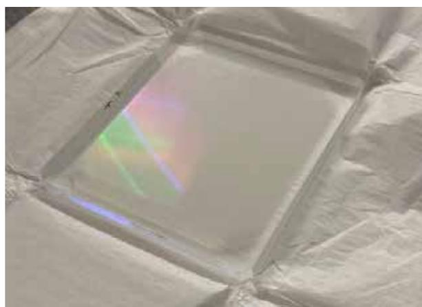
The new 700 l/mm VPH grating for the RSS being unwrapped in the lab.
