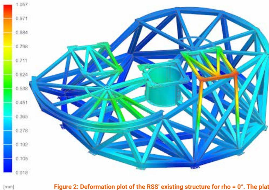
**Figure 2: Deformation plot of the RSS' existing structure for  $\rho = 0^\circ$ . The platform on the right, which houses the VIS electronics cabinet, shows a maximum deflection of just over 1 mm in this orientation.**
