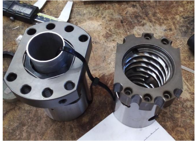
A new ball screw (left) and the wire cut and spark eroded ball screw nut housing (right).
