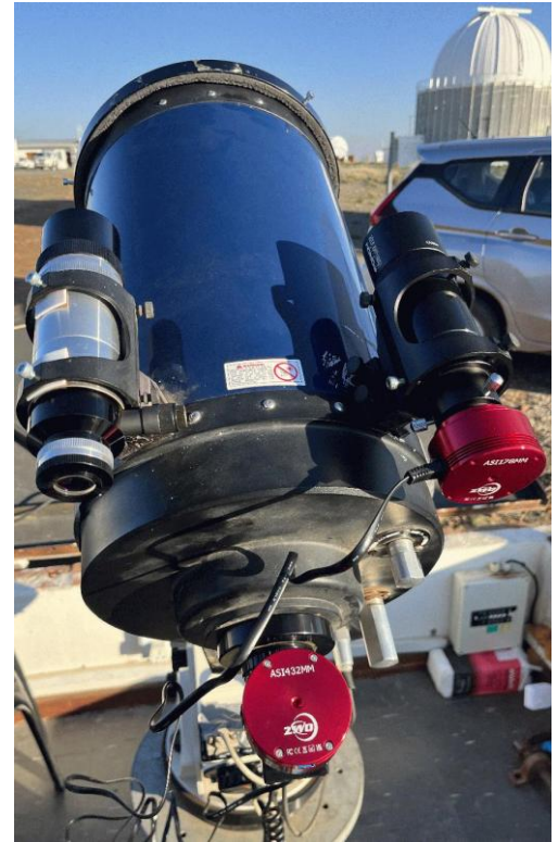
The telescope with the new seeing camera at the bottom and new acquisition camera to the right (both in red).
