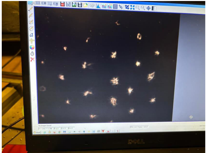
SPIFFY image from the CCAS tower, showing defocused return spots from individual segments after bursting the array.
