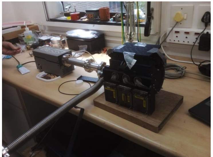
RSS Cryostat re assembled and under vacuum with the RGA connected to check the vacuum integrity after the fix.
