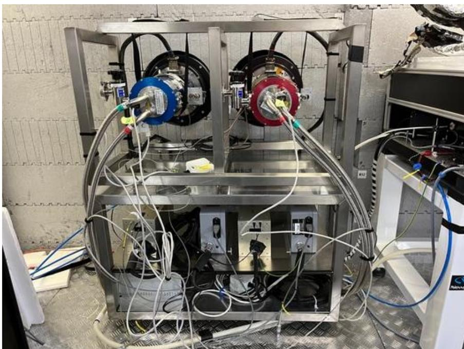
HRS cryostats, prior to disconnection from the vacuum tank on 31 January.
