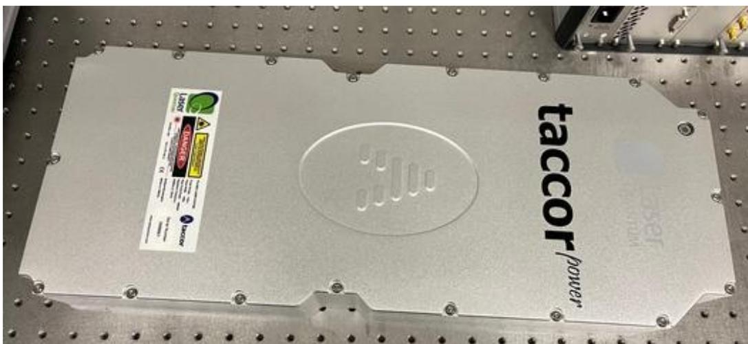
The 800 nm Ti:Sapphire femtosecond pulsed laser that will drive the LFC.
