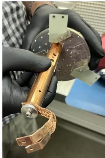
New flexible copper braid at the CCD-end of the Red cryostat's cold-finger.
