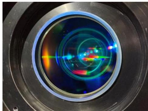
Full-colour echellogram visible when illuminating the HRS Red camera optics.
