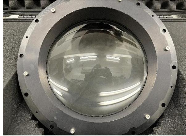
The current RSS collimator triplet (left) with its coupling fluid drained out, showing the problematic residues from the original fluid. When the triplet is filled with fluid, these structures are greatly reduced, but the scattering produced by this random array of "micro-lenses" certainly reduces the signal-to-noise in RSS data. The image on the right shows the new collimator triplet, filled with pristine lens fluid.
