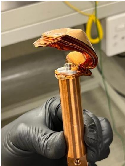
Copper leaves at the CCD-end of the Red cryostat's cold-finger.
