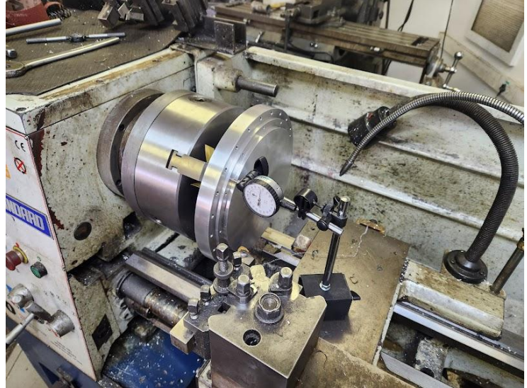
Left: One of the main group shims. Right: The jig for machining the main group shims being set up on the lathe in the SALT workshop.
