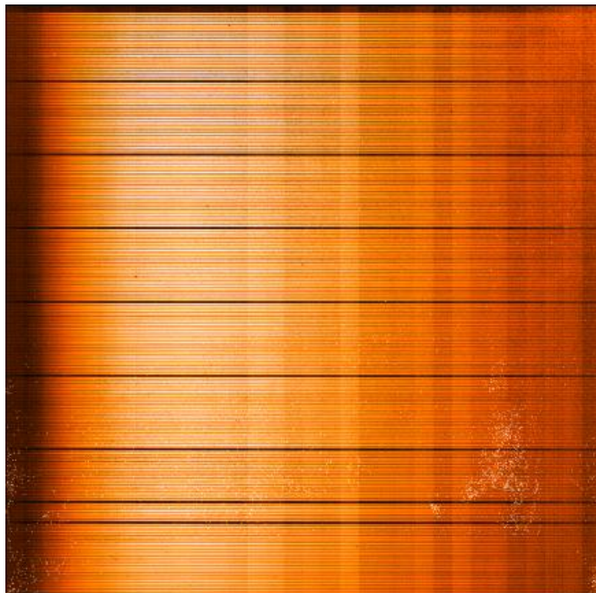
First calsys light through the instrument (7 July, 01:42). This was taken using the QTH2 lamp and optical lightguide and with the instrument setup at the bluest grating angle. The light from all 248 fibres is seen on the detector.
