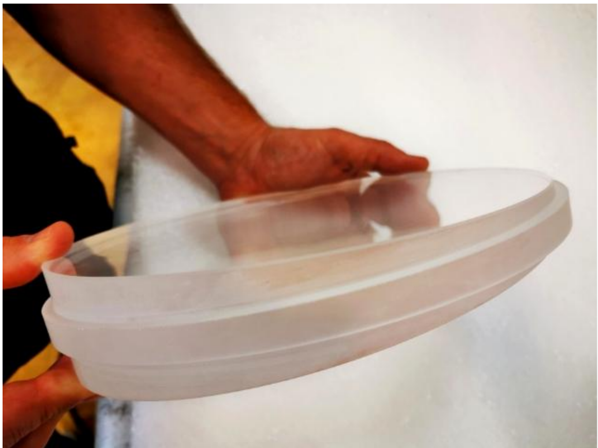
Figure 2 Lens after CNC machining
