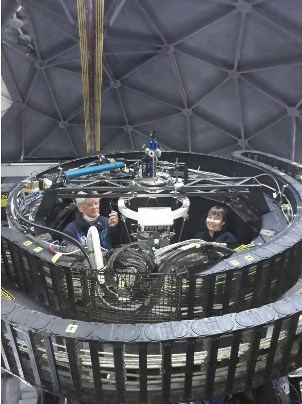
Francois and Melanie in the normal payload position doing the optical alignment measurements between the SAC and the Rho stage of the tracker.
