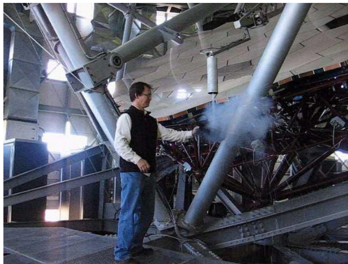
Well dressed SALT Mechanical Engineer, Ockert Strydom, inspects the CO 2 mirror cleaning system nozzle during commissioning tests in 2008.
