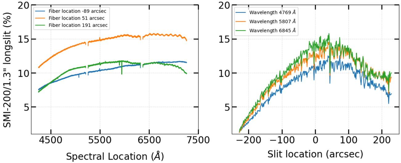
**Figure 3:** Measured SMI-200 relative throughput compared to 1.3 arcsec longslit in different (left) spatial locations and (right) spectral channels. The used configuration was 30.25 degree camera and 15.125 degree grating angle (PG900).
