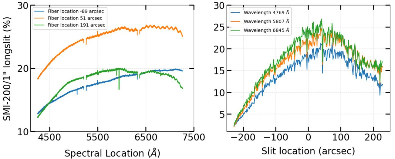
**Figure 4:** Estimated SMI-200 relative throughput compared to 1 arcsec longslit in different (left) spatial locations and (right) spectral channels. The used configuration was 30.25 degree camera and 15.125 degree grating angle (PG900).
