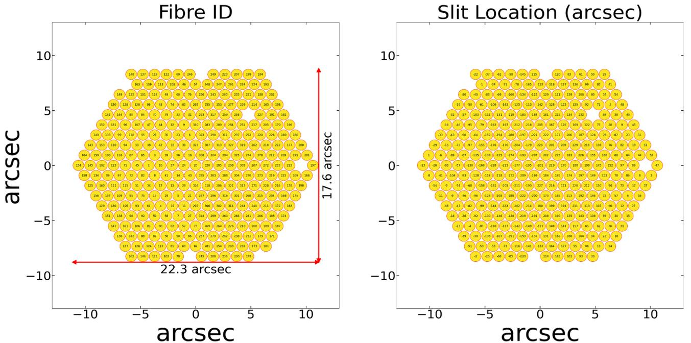
**Figure 2:** X and Y axis denote location of fibres on the sky. The annotated numbers inside each fibre footprint defines (right) the location of the same fibre at the slit which is at the input of the spectrograph in arcsec where 0 arcsec is the centre of the slit; and (left) the ID of the same fibre at the slit where 1 and 327 denote the lower end upper end fibre respectively.
