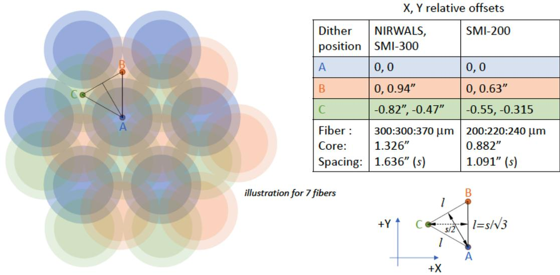
**Figure 5:** Dither pattern of the SMI-200 fibres to obtain truly integral field coverage. One may use 1/3rd of the total exposure time at each dithered location.
