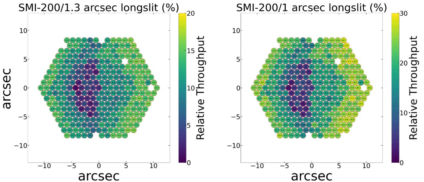
**Figure 5:** On-sky relative throughput distribution of SMI-200 compared to the 1.3 arcsec longslit. Use the right panel throughput to estimate the additional exposure time required compared to RSS simulation tool with 1 arcsec slit. Multiply the RSS simulated exposure time with  $\sqrt{100/\text{fibre throughput}}$  to obtain the required exposure time.
